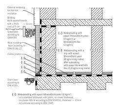
> Waterproofing against water pressing from the inside according to DIN 18195-7
